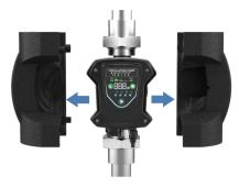
The water pump foam for the heating system is attached with the pump. Before installing the water pump, remove the heat insulating foam, and then put the foam on the pump body after the installation is completed.
